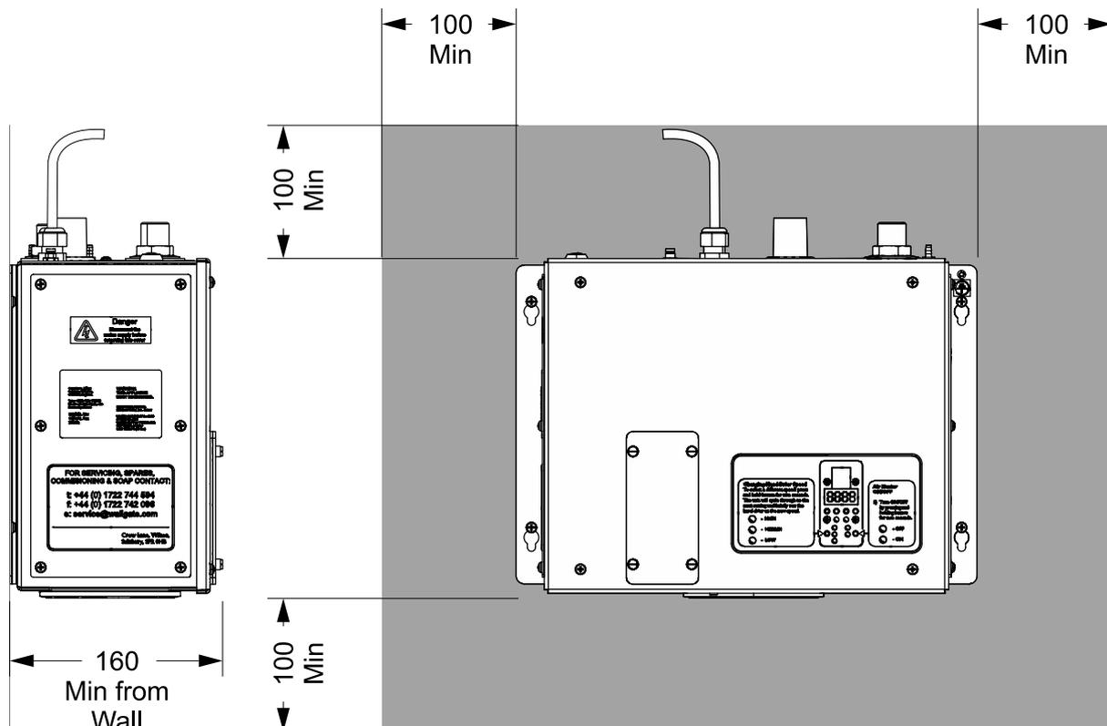
Ensure adequate ventilation to the bottom of the engine
