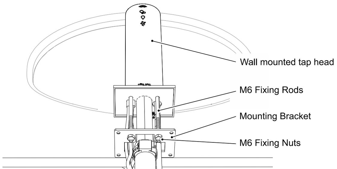
**Figure 9:** Rear view tap head installation into wall.
