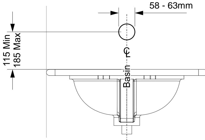
**Figure 3:** Wall Mounted Tap Head mounting dimensions.
