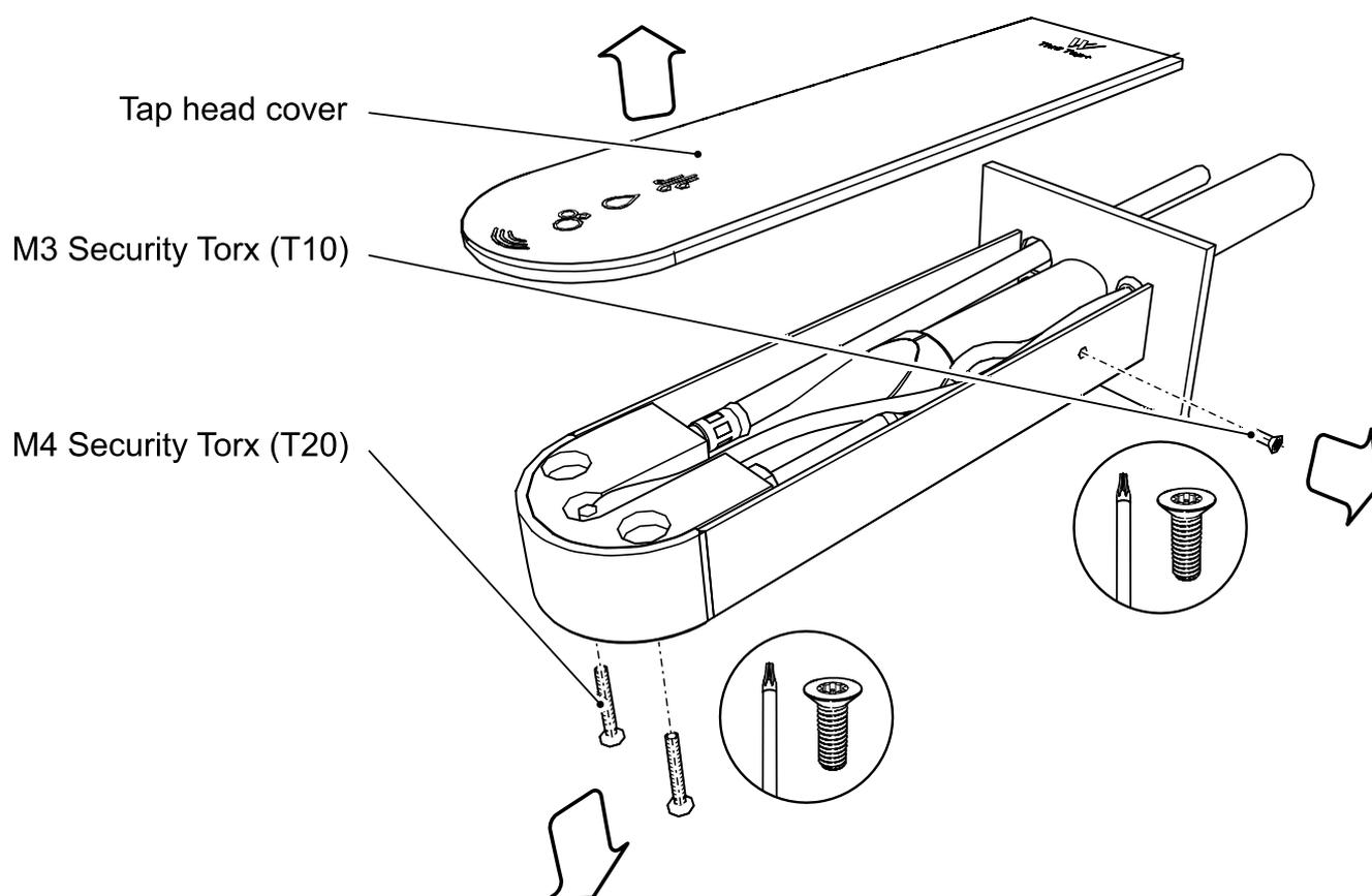
**Figure 11:** Front fix wall mounted tap head assembly.
