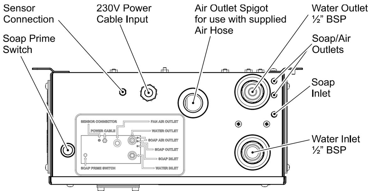
**Figure 15:** Control Module I/O arrangement.
