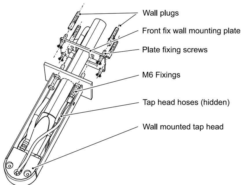
**Figure 13:** Front fix wall mounted tap installation.
