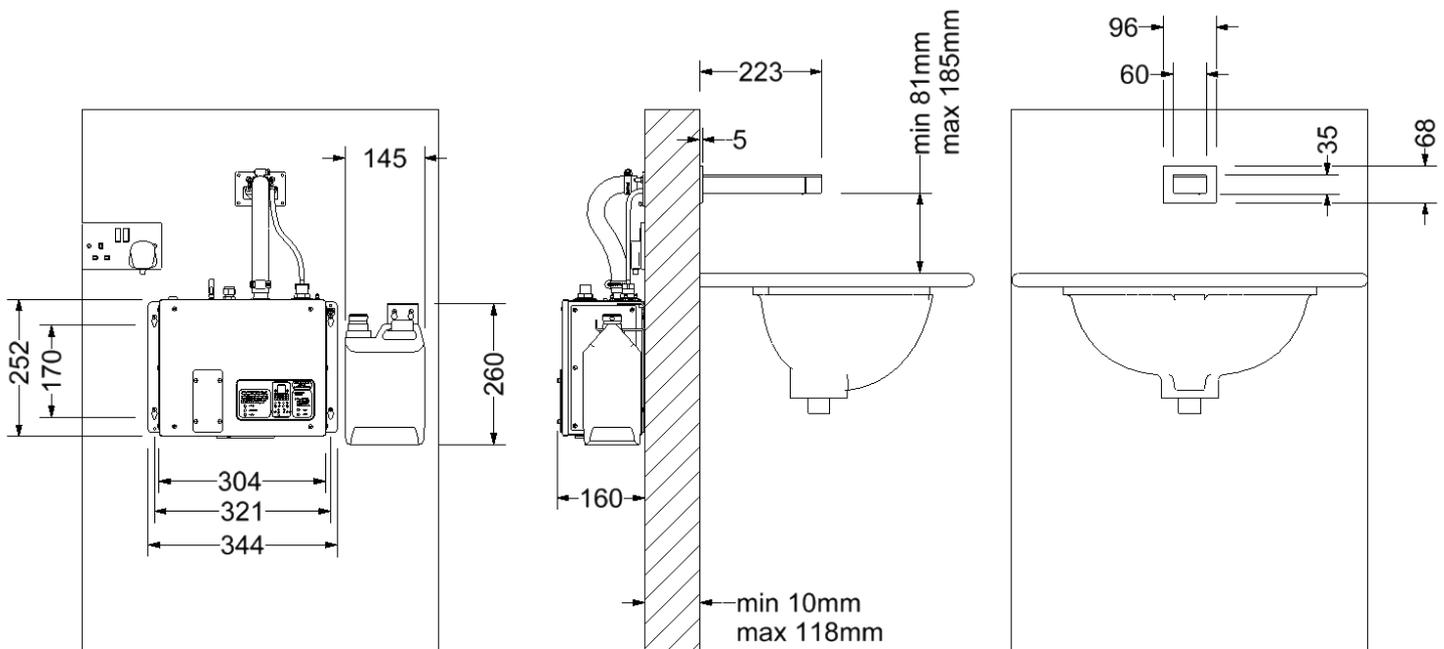
**Figure 1:** Wall mounted tap dimensions [mm]
