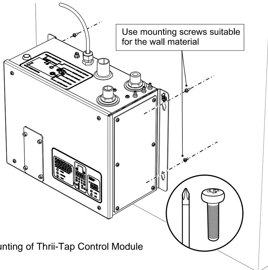
**Figure 5:** Wall mounting of Thrii-Tap Control Module
