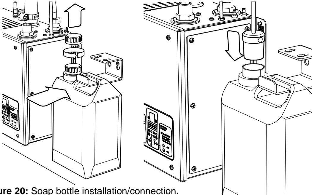
**Figure 20:** Soap bottle installation/connection.
