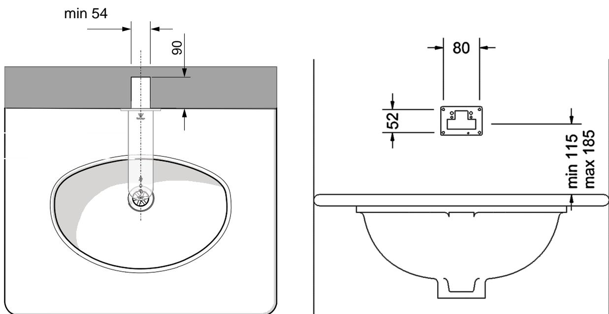
**Figure 4:** Front Fixed Wall Mounted Tap Head mounting dimensions.
