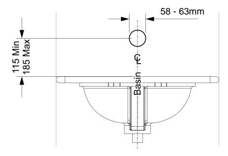
Figure 3: Wall Mounted Tap Head mounting dimensions.
