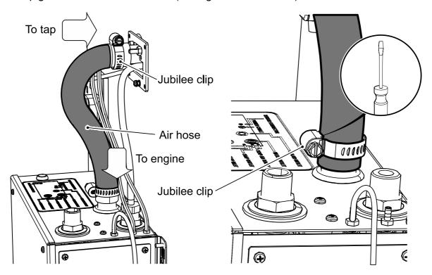
Figure 16: Air hose connection.
