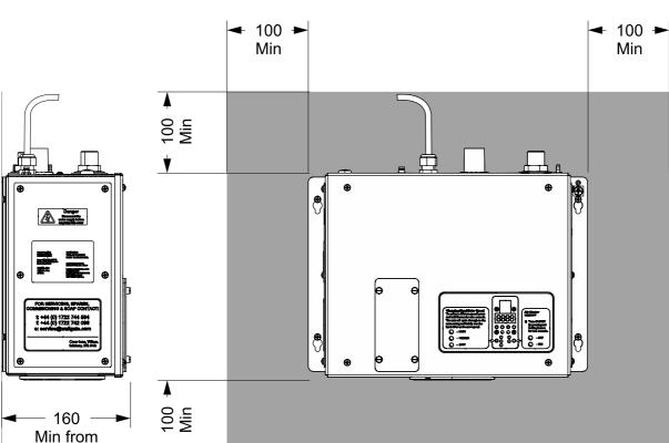
The module must have a clearance envelope of 100mm (see Fig 6).
