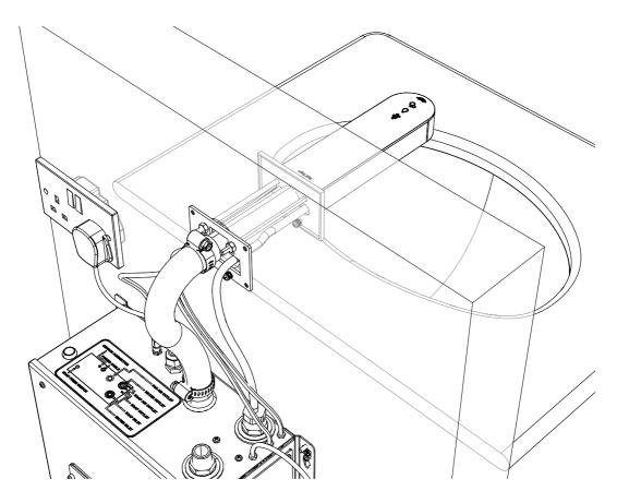
Figure 10: Complete wall mounted tap head installation (rear fixing).
