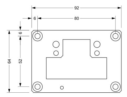
Figure 12: Front fix wall mounting plate.
