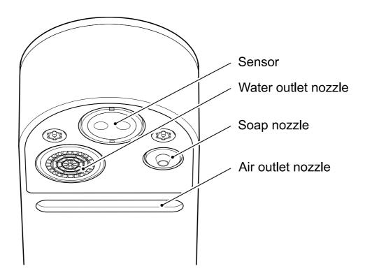
Figure 2: Tap head outlet nozzles.
