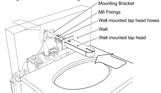
Figure 8: Front view tap head installation into wall.
