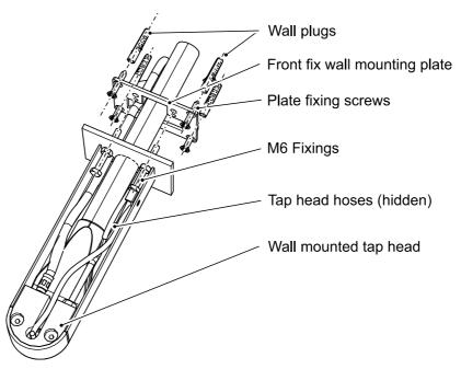
Figure 13: Front fix wall mounted tap installation.
