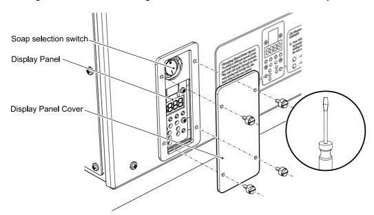
Figure 22: Display cover removal.
