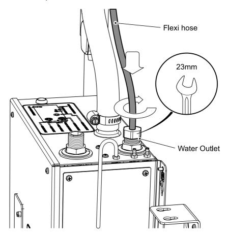
Figure 17: Flexi hose / water outlet connection
