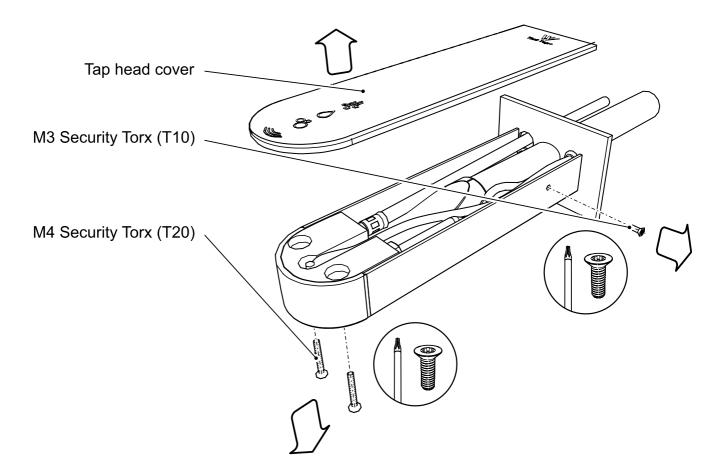
Figure 11: Front fix wall mounted tap head assembly.
