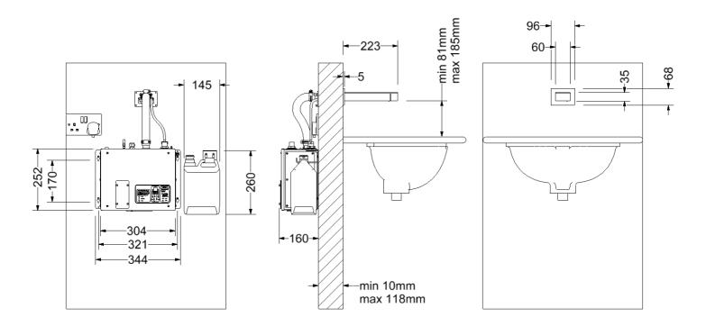
Figure 1: Wall mounted tap dimensions [mm]
