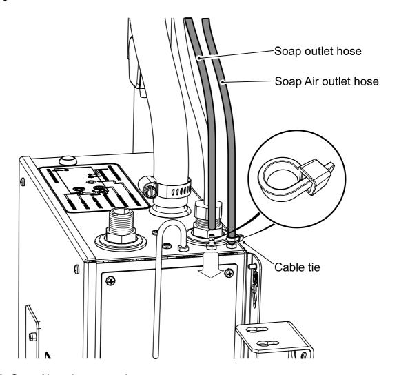
Figure 19: Soap Air outlet connections.
