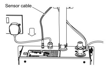
Figure 18: Sensor cable connection.
