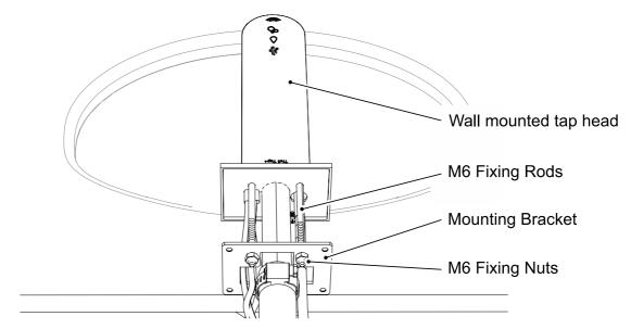
Figure 9: Rear view tap head installation into wall.
