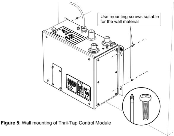
The control module can be mounted either with the inputs and outputs pointed downwards for through wall installations, or upwards for both through wall and under basin installations.
