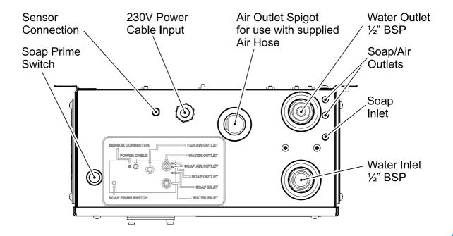
Figure 15: Control Module I/O arrangement.
